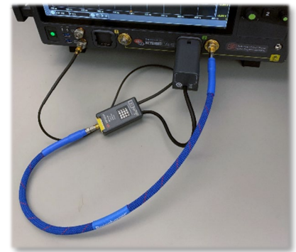
PrecisionProbe characterization of a 1.85 mm cable to 70 GHz using the N2126A optimization module
